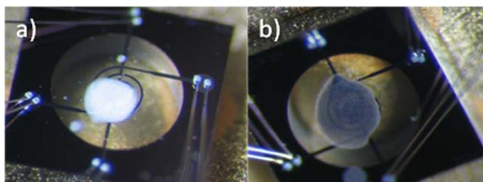
Figure 1: New gas sensor devices coated with a) undoped nanosized SnO<sub>2</sub> and b) Pt doped nanosized SnO<sub>2</sub> thick layers
