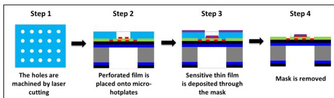
FIGURE 2: Integration process of  $\text{ZnO:Ga}$  using stencil mask.
