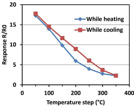
FIGURE 9: Response of ZnO:Ga as a function of the temperature step (step duration is 5 minutes).
