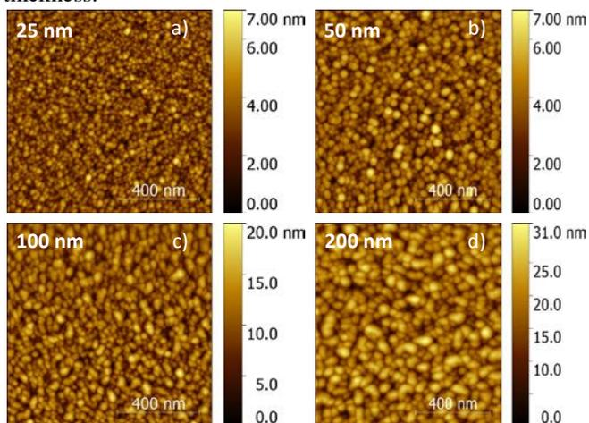
FIGURE 5: AFM micrographs of a) 25 nm, b) 50 nm, c) 100 nm and d) 200 nm thick ZnO:Ga thin films.
