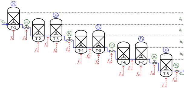
Fig. 1. Diagram of the flotation process under study.
