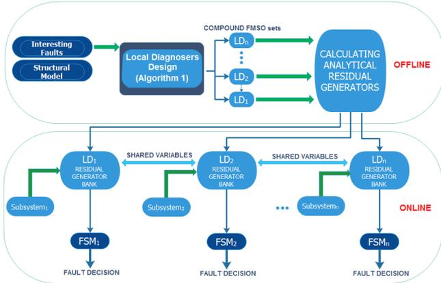
Fig. 3. Scheme of distributed generation of LDs.
