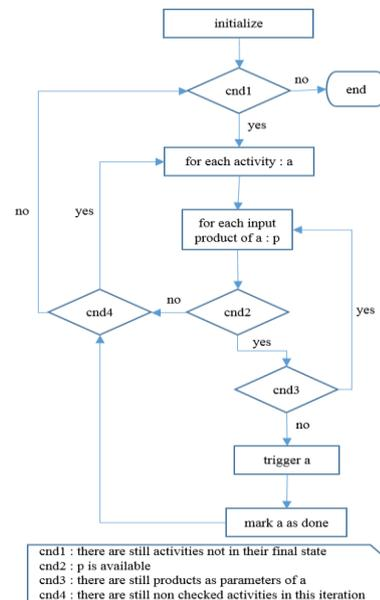
Figure 5. Flow execution of synchro state process aspect.
