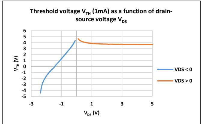
Fig. 7. Threshold voltage  $V_{TH}$  as a function of the drain-source voltage  $V_{DS}$  (here, the threshold voltage is defined as the minimum value of the gate bias voltage that allows a current of 1mA accros the MOSFET at a fixed drain-source voltage).
