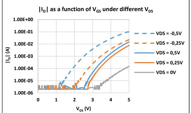
Fig. 6. Transfer characteristics of SiC MOSFET (in logarithmic scale) under different drain-source voltages
