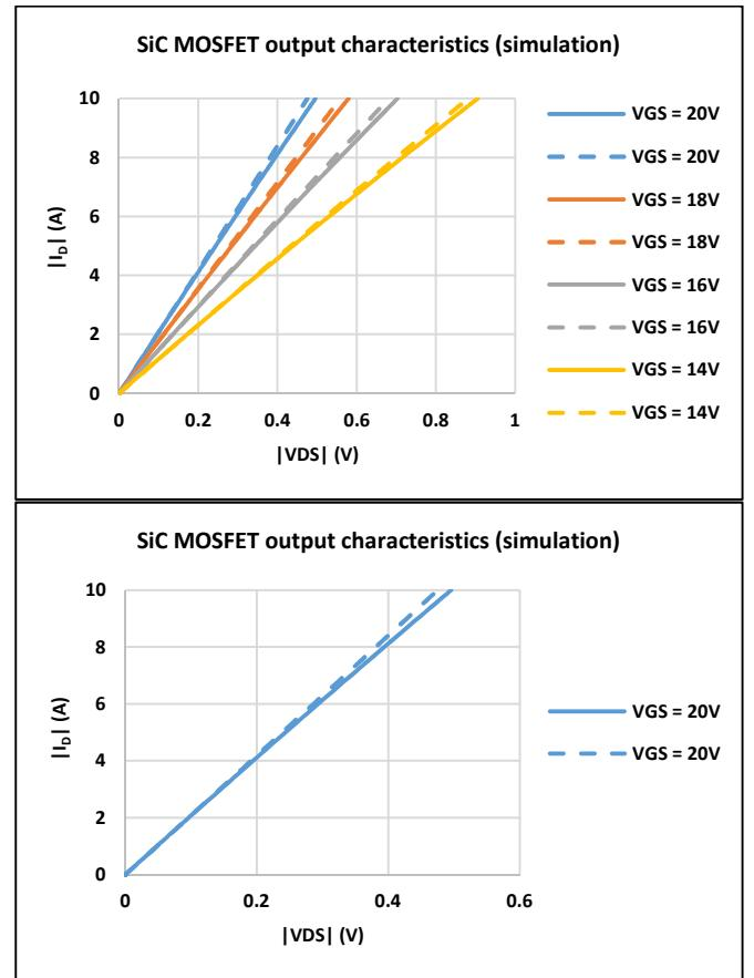
Fig. 3. Comparison of simulation forward and reverse output characteristics of STM SiC MOSFET (SCT50N120) under the gate bias voltage  $V_{GS} = 14-20V$  and a zoom for  $V_{GS} = 20V$  (reverse conduction as dashed line, forward conduction as continue line).
