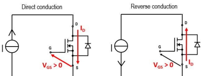
Fig. 1. Measurement circuit of SiC MOSFETs: forward (direct) conduction and reverse conduction.
