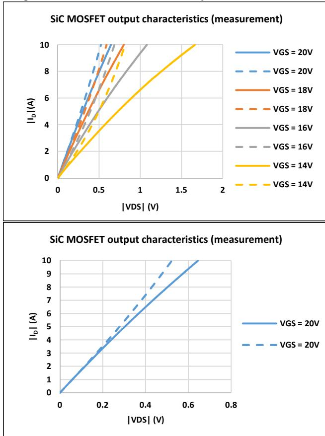
Fig. 2. Comparison of measurement forward and reverse output characteristics of STM SiC MOSFET (SCT50N120) under the gate bias voltage  $V_{GS} = 14-20V$  and a zoom for  $V_{GS} = 20V$  (reverse conduction as dashed line, forward conduction as continue line).
