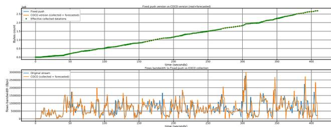
Fig. 6. Bandwidth Estimated from the bytes count collected
