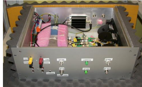
Fig. 1. Optical FM noise measurement system: 2 km delay line frequency discriminator with 80 MHz frequency offset obtained with an acousto-optic modulator. The output signal at 80 MHz is measured on a E5052B RF phase noise analyzer.
