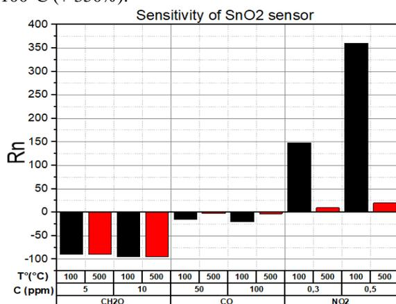
**Fig. 1.** Response of SnO<sub>2</sub> gas sensors operated with pulsed temperature modulation in different gaseous environment
