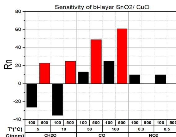
**Fig. 3.** Response of Bi-layer SnO<sub>2</sub>/CuO sensor gas sensors operated with pulsed temperature modulation in different gaseous environment
