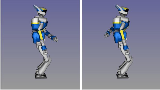
Fig. 9. Constrained motion planning for HRP-2 humanoid robot sliding on the ground in quasi-static equilibrium: the feet should stay horizontal with a fixed relative position and the center of mass should project between the feet. The initial configuration is shown on the left. The goal configuration is shown on the right. The algorithm is a constrained RRT close to the one described in Dalibard *et al* [16].
