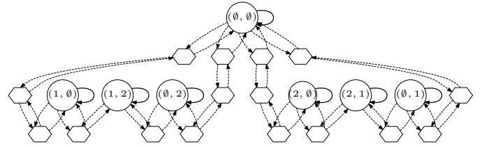
Fig. 7. Structure of the constraint graph corresponding to the system in Section V-D2 after inserting waypoint transitions. Waypoint transitions starting from/going to  $(0,0)$  contain three waypoint states. All other waypoint transitions contain one waypoint state.
