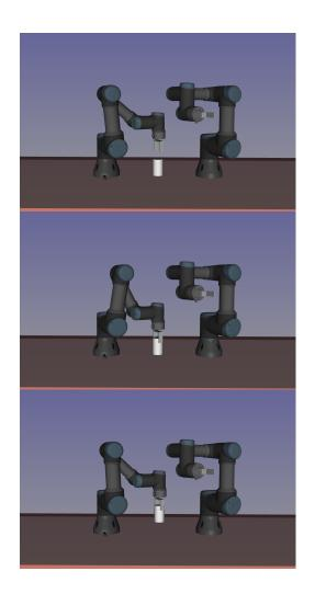
Fig. 8. Example of extension along the waypoint transition between states  $(\emptyset, \emptyset)$  and  $(1, \emptyset)$ . Each picture represents a waypoint. The last waypoint is in state  $(1, \emptyset)$ .  $\mathbf{q}_{near}$  and  $\mathbf{q}_{rand}$  are the same as in Figure 3.
