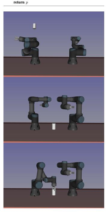
Fig. 3. Example of extension along a transition of the constraint graph. Top  $\mathbf{q}_{rand}$ , middle  $\mathbf{q}_{near}$ , bottom  $\mathbf{q}_{target}$ .
