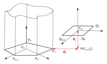
Fig. 2. Distance defined by two convex polygons.
