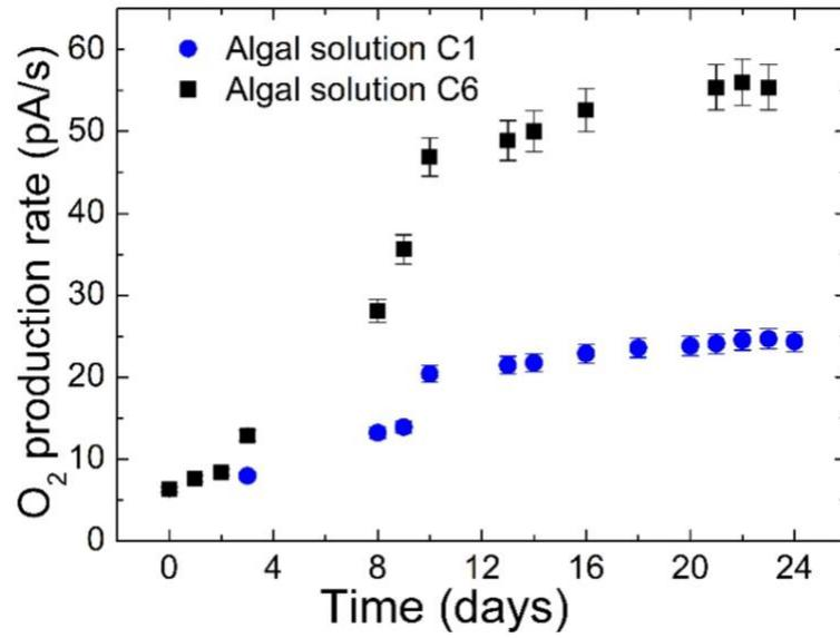
Figure 4: Temporal variations of the oxygen production rate of fresh algal solutions (C1: pristine solution and C6: six-times concentrated solution, culture illumination: 30 cd/m<sup>2</sup>)
