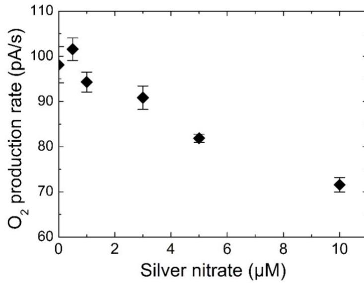
Figure 7: Evolution of the oxygen production rate with silver nitrate concentration
