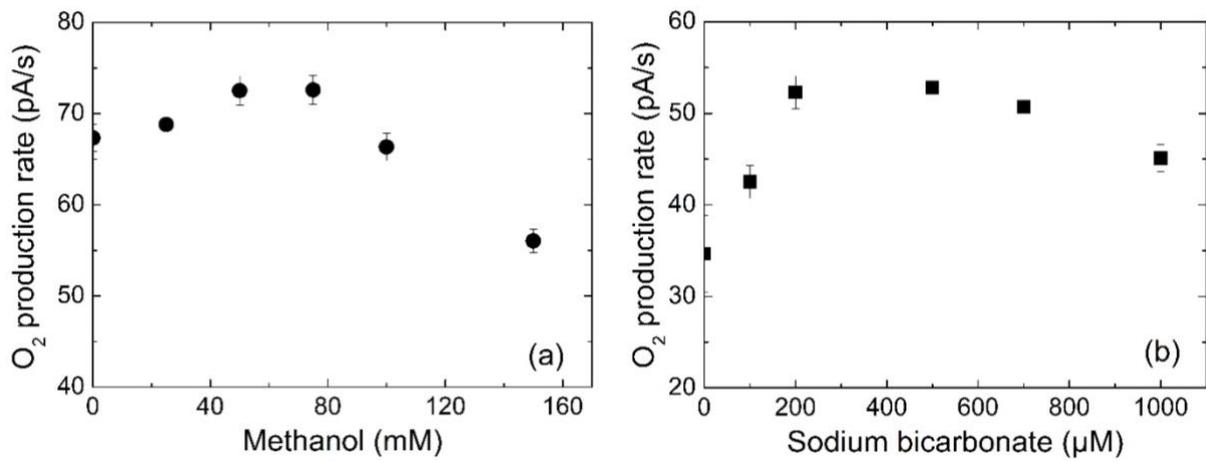
Figure 5: Evolution of the oxygen production rate with carbon nutrient concentration for the pristine solution C1: left) methanol  $\text{CH}_3\text{OH}$  and right) sodium bicarbonate  $\text{HCO}_3\text{Na}$ . All data are mean experimental values and error bars are calculated standard deviations.
