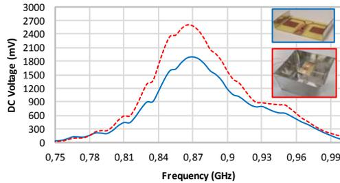
Figure 7: Measured dc voltage for the two manufactured rectennas as function of the frequency in an anechoic chamber. RMC (red dashed line) and RT (continuous blue line) at a power density of  $3.4 \mu\text{W}/\text{cm}^2$ .
