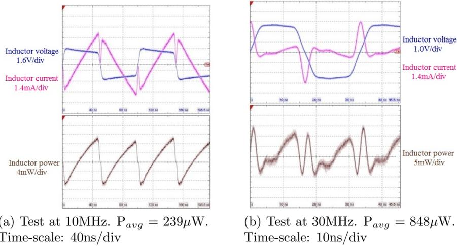
Figure 15: Test inductor SRP5015A at 10MHz and 30MHz.
