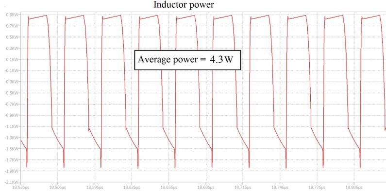
Figure 6: Inductor power in the time-domain.
