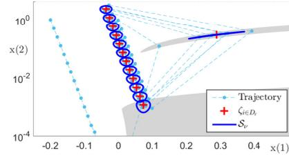
Fig. 7. Example 3: Trajectories of (27)-(28) obtained for a perturbation  $\delta_{max} = 0.01$ . The grey areas correspond to the regions of the state space, where the control law imposes to select mode 2.
