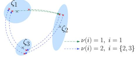
Fig. 2. Schematic representation of a robust limit cycle associated to a cycle  $\nu$  of period  $N_\nu = 3$ , for a system (1) with  $K = 2$  modes.
