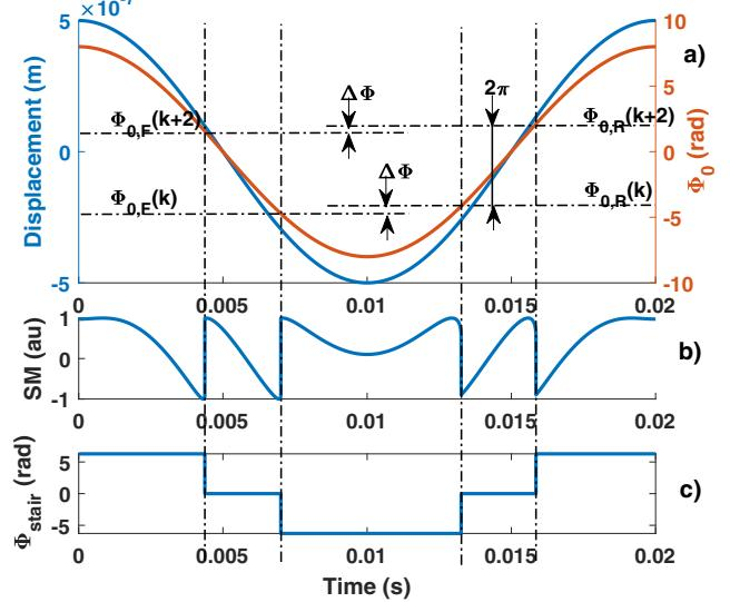
Fig. 2. Simulated typical Self-Mixing signal (b) obtained for (a) a  $0.5\mu\text{m}$  sinusoidal displacement, a laser wavelength  $\lambda_0=785\text{ nm}$  and  $C=1.5$  (in blue line) with its corresponding phase  $\Phi_0$  (in red) and (c) staircase phase  $\Phi_{stair}$ .
