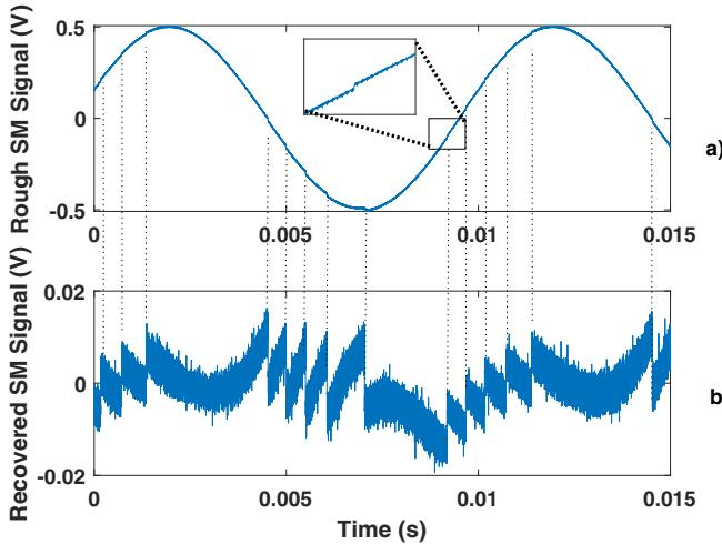
Fig. 3. Measured rough SM signal (a) obtained for a target vibrating at  $f_v = 10$  Hz with a 150 nm amplitude. A dithering current signal modulates the LD drive current at 100 Hz. Note that the optical output power is directly modulated by the LD current dithering signal. In (b), recovered SM signal from a) after filtering out the dithering signal.
