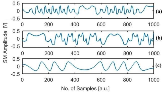
Fig. 1. Experimental multi- (a-b) and mono-modal (c) SM signals acquired under different optical feedback coupling and operating current conditions based on HL6501MG LD ( $I_{th}=45\text{mA}$ ) with  $I_{oper}$  of (a-c) 78 mA, and (b) 82 mA.
