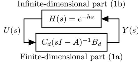
Figure 1: Block diagram of time-delay system (1).
