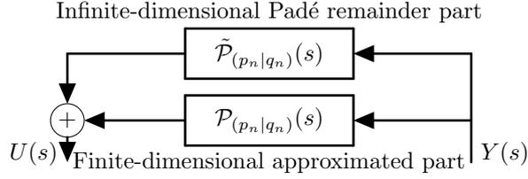
Figure 2: Naive modeling of the delay element (1b).
