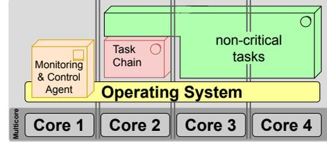
Fig. 3. Monitoring & Control Agent basic concept
