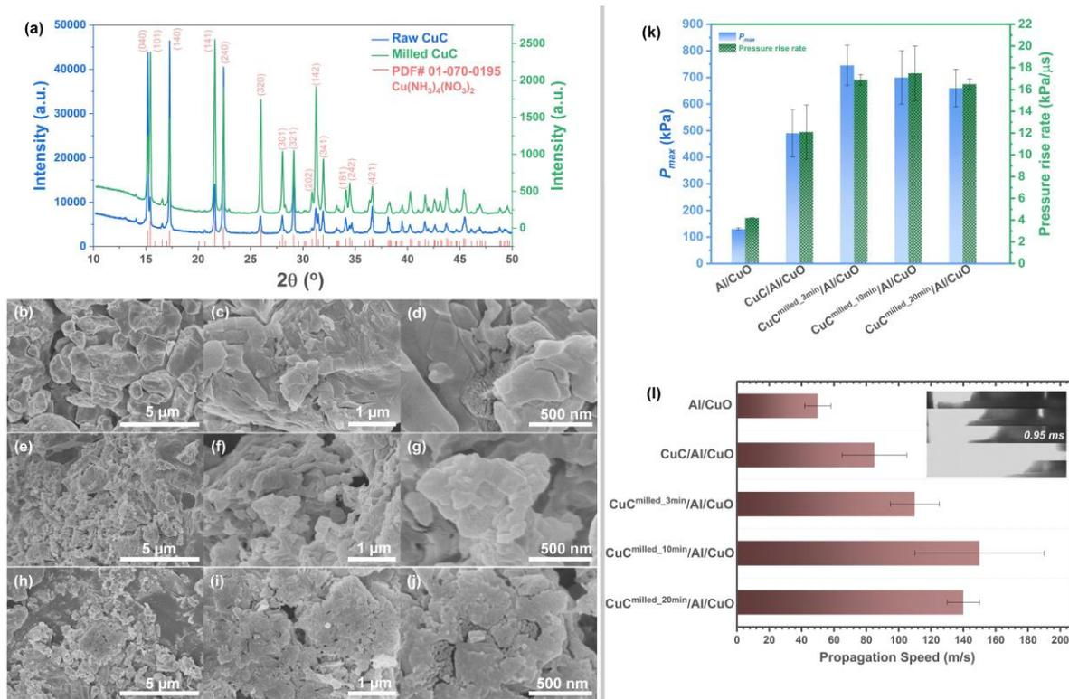
**Figure 1.** (a) XRD patterns of milled CuC in comparison to raw CuC; SEM images of CuC milled by 3 (b-d), 10 (e-g), and 20 minutes (h-j); maximum generated pressure and pressure rise rate (k), and propagation speed results (l) of different CuC/Al/CuO RMs. The inset image in (l) is a snapshot from the propagation test videos of these five materials at 0.95 ms (see supplement, **Video S1**).
