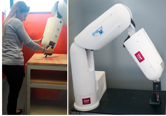
Fig. 1: (Left) Experimental setup for user study. (Right) ISybot 6-DOF Collaborative robot.
