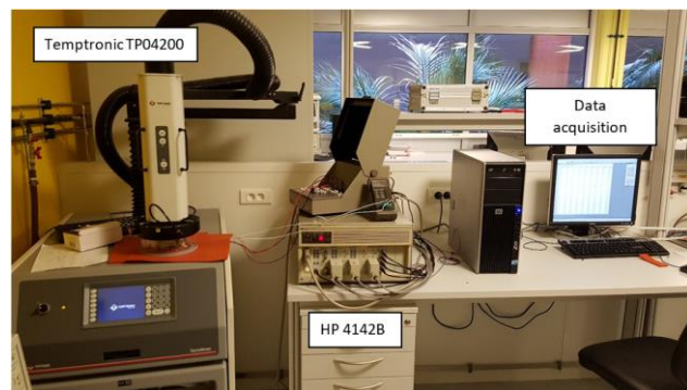
Fig. 3. Electrical test bench for power module characterization.
