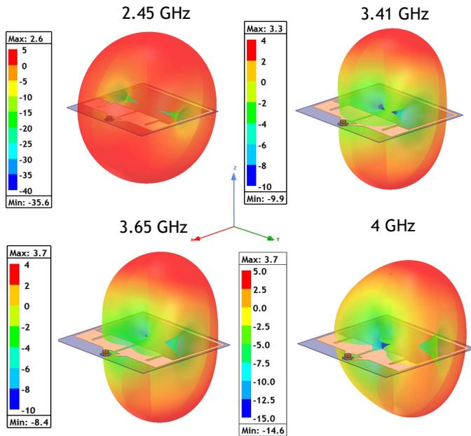
Fig. 7. Simulation of the 3D radiation pattern of the proposed antenna at different frequency.
