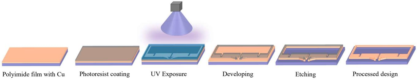
Fig. 9. Schematic representation of the photolithographic process.
