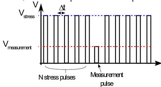
Fig. 4. Sequence of stress and measurement pulses
