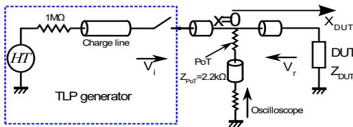
Fig. 1. Schema of TLP-based TDR measurement method
