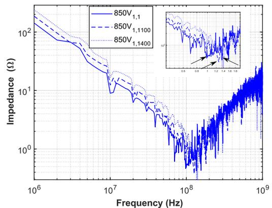
Fig. 8. Complex impedance of the X7R capacitor after
