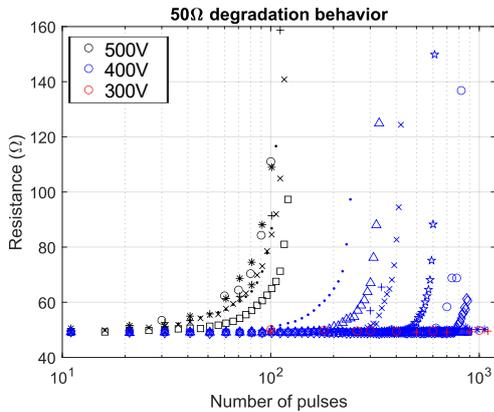
Fig. 5. 50  $\Omega$  resistance degradation according to the number of TLP stress from 300 V to 500 V
