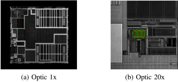
Fig. 2: Laser picture of the SAM3X8E
