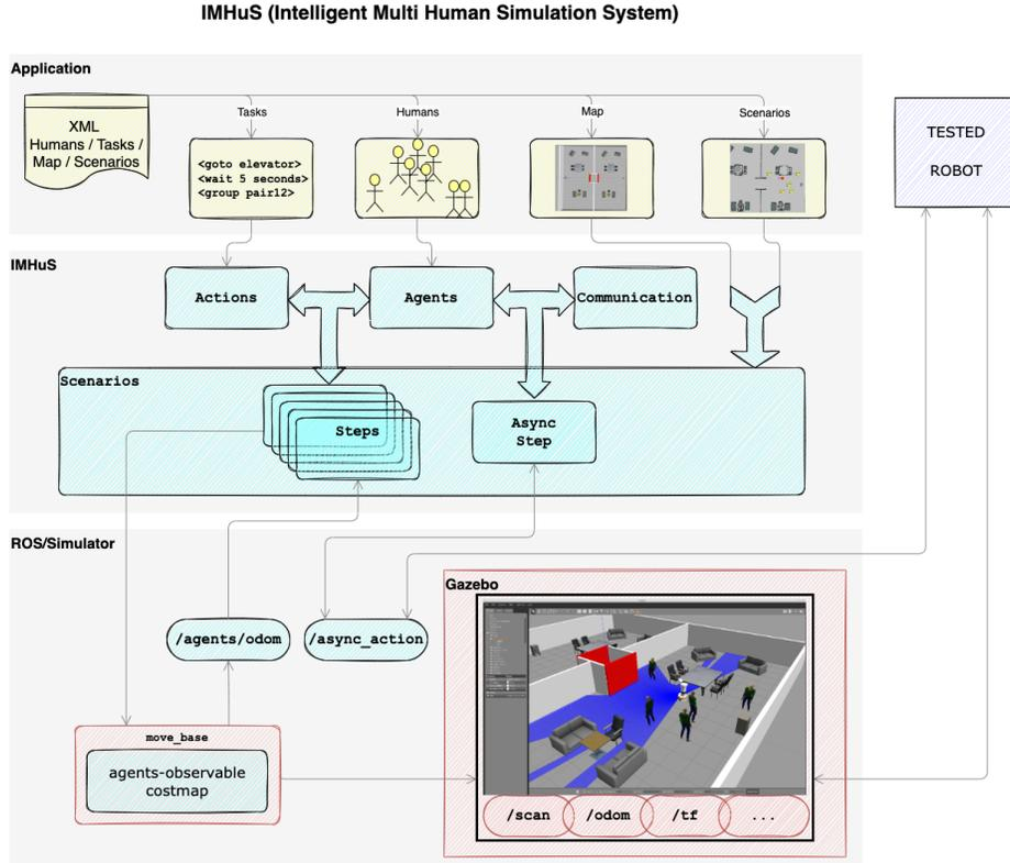
**Fig. 4.** Structure of the new IMHuS tool.
