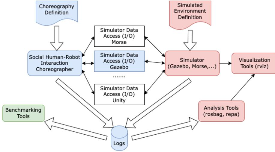
**Fig. 3.** Global simulation architecture. Red signifies existing tools, blue components are those described in this paper, green signifies on-going development, and uncolored boxes alternative simulators under consideration.
