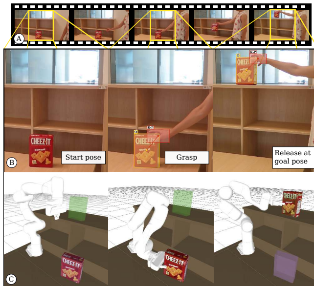
Fig. 1. The proposed planning approach is guided by the demonstration video (A). The video depicts a person manipulating a known object; the cheez-it box in this particular example. The video can contain several pick-and-place actions with multiple objects. Here only a short clip with only one object and one action is shown. From the video we recognize (i) the contact states between the human hand and the object, marked by red bounding boxes in (B); and (ii) the object 6D pose (3D translation and 3D rotation w.r.t camera) at the grasp and release contact states, marked in yellow in (B). The robot trajectory planned by the proposed approach is shown in (C). The start and goal object poses in (C) are shown in magenta and green, respectively.
