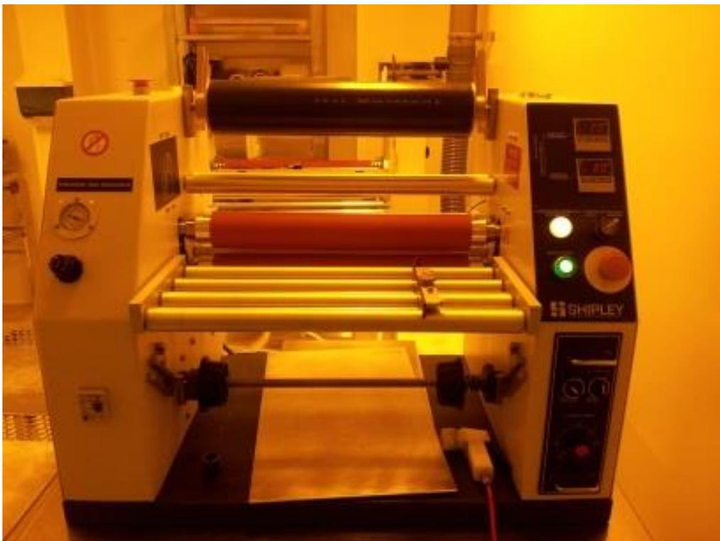
Figure III.3: Shipley 360N Laminator.
