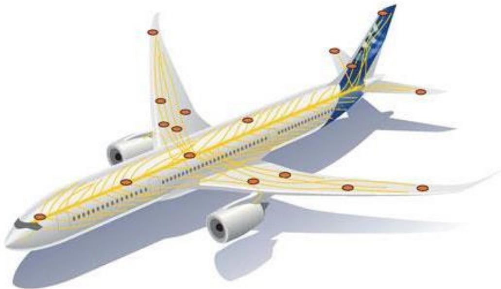
Figure I.1: Structural health monitoring (SHM) systems arrayed in key areas where loads are highest. Source: Airbus
