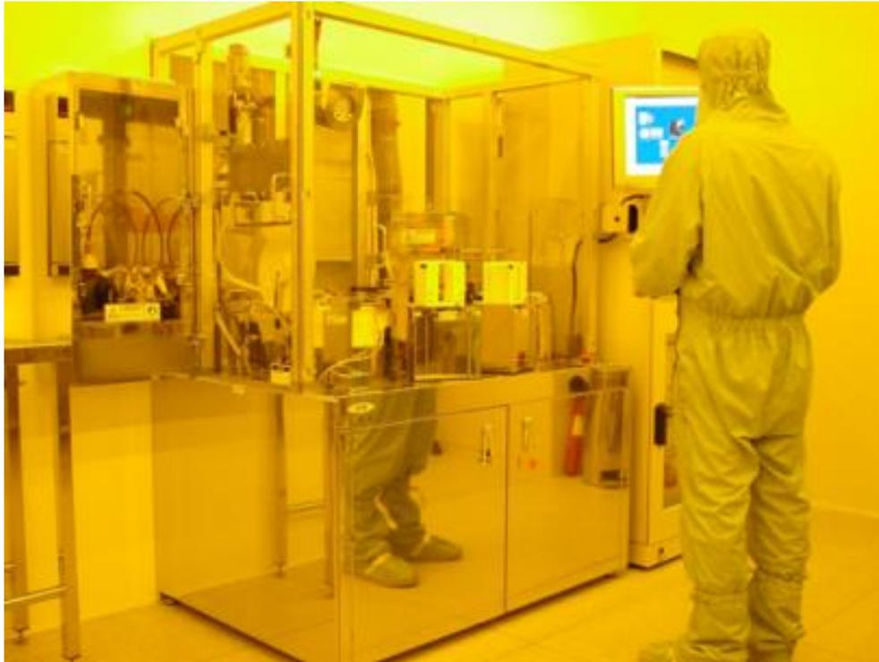
Figure III.4: EVG120 resist processing system.
