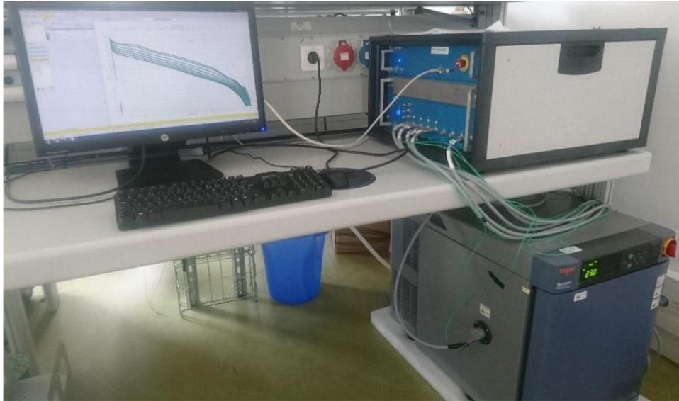
Figure 3.22 Experimental setup for cycling batteries
