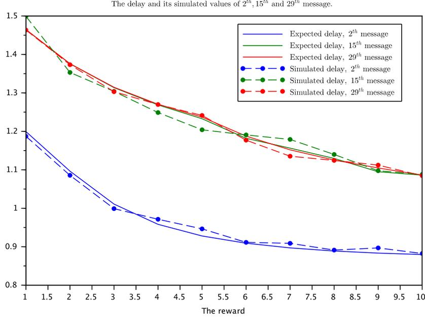
Figure 3.9: Comparison of the theoretical expected delays of 2<sup>nd</sup>, 15<sup>th</sup> and 29<sup>th</sup> messages against expected delays obtained through simulations.
