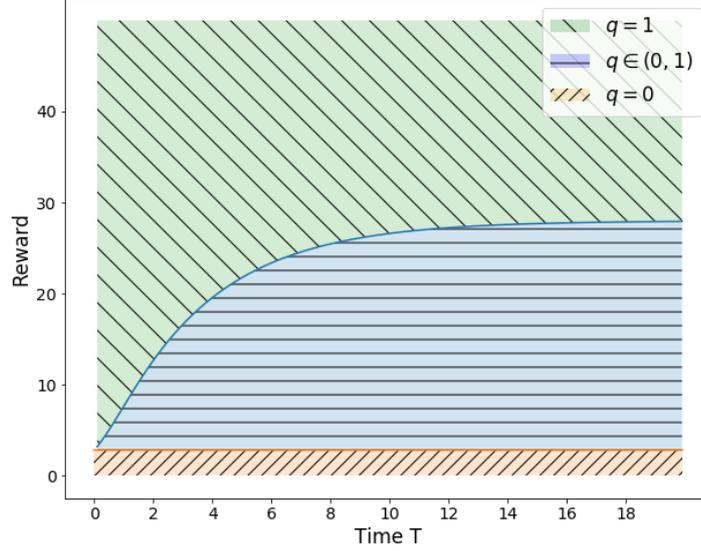
Figure 5.1: Equilibrium acceptance probability  $q_1$  as a function of  $R$  and  $T$ , when the values of the parameters are as follows:  $\mu = 0.5$ ,  $\lambda = 0.3$ ,  $C_r = C_d = 2$  and  $C_s = 0.4$ .
