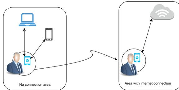
Figure 1.7: In areas where there is no network connectivity, nodes forward data to relays who may move to connected areas. Once a relay has an Internet connection, it sends data to a server.
