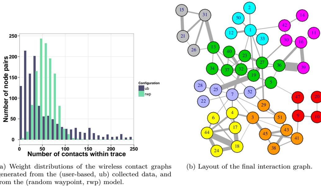
(a) Weight distributions of the wireless contact graphs generated from the (user-based, ub) collected data, and from the (random waypoint, rwp) model.
