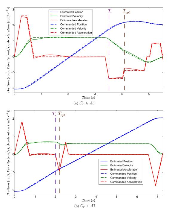
Figure 3.15: Illustration of motion constraints abrupt switch on a KUKA-LWR4 joint axis.
