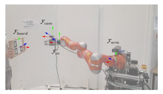
Figure 3.19: Visual servoing experiment (see [video-2]). The arm's end effector is following the wooden board. The board is tracked by a Kinect camera placed on its gripper.
