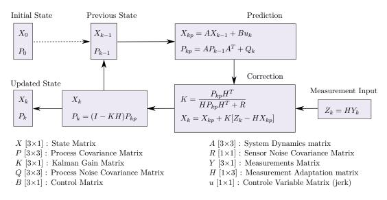
Figure 3.10: Depiction of a Single Dimensional Kalman Filter used to estimate the current angular state of the Kuka arm (Fig. 3.12).
