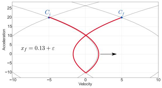
(b) Positive loop trajectory corresponding to the situation depicted by the blue circle on the timeoptimal curve  $C_{opt}$  of Fig. 2.10.
