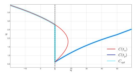
Figure 2.8: A shift of the initial and final velocities distort the curves  $C(t_n)$  and  $C(t_p)$ . It can be noted that the curve  $C_{opt}(x_f)$  has a discontinuity for  $x_f = \lambda$ .  $(J_{min} = -50, J_{max} = 50, A_{min} = -30, A_{max} = 30, V_{min} = -30, V_{max} = 30, a_i = 8, v_i = 10, a_f = 8, v_f = 20).$
