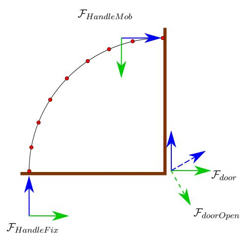
Figure 4.8: With the relations between the frames depicted in Fig. D.2, we express the coordinates of each frame relatively to others according to the opening angle of the door. By repeating the process with different opening angles we can obtain a series of  $\mathcal{F}_{EE}$  expressed in  $\mathcal{F}_{Arm}$ . From there we can compute a via-points trajectory describing the door's opening.
