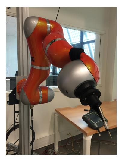
Figure 3.12: A KuKa LWR4 robotic arm used for our experiments.
