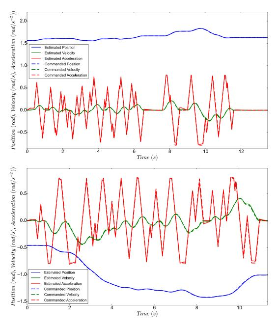
Figure 3.22: Evolution of angular trajectories during some visual servoing experiments. As the trajectory planner runs at 10Hz, trajectories are replanned multiple times while the robot is moving. Junction trajectories are used to smooth the trajectories switch.
