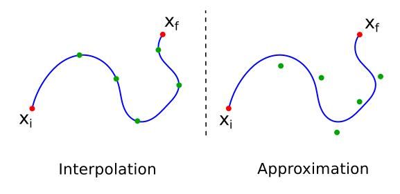
Figure 1.15: Differences between interpolation and approximation.
