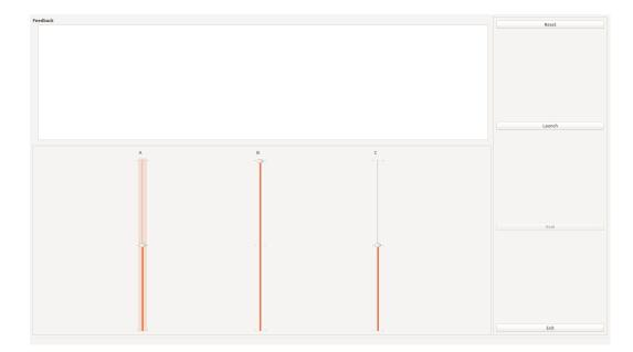
Figure 4.1: Screen shot of the interface used by the participants to set the kinematic bounds. A was for acceleration, B for jerk, C for speed. Participants didn't had this information. We can also see a launch button used to begin a new test, and an eval button that opens a new Godspeed questionnaire to fill.
