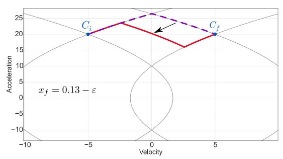
(a) Positive shortcut trajectory corresponding to the situation depicted by the golden circle on the time-optimal curve  $C_{opt}$  of Fig. 2.10. From the direct trajectory we increased  $x_f$  until we reach a discontinuity on  $C_{opt}$ . By increasing  $x_f$  more we leave the lens shaped curve of 2.10 and the trajectory will now be a positive loop that can be extended indefinitely. See (b).
