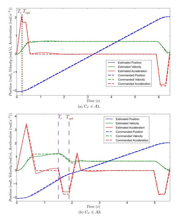
Figure 3.14: Illustration of motion constraints abrupt switch on a KUKA-LWR4 joint axis.
