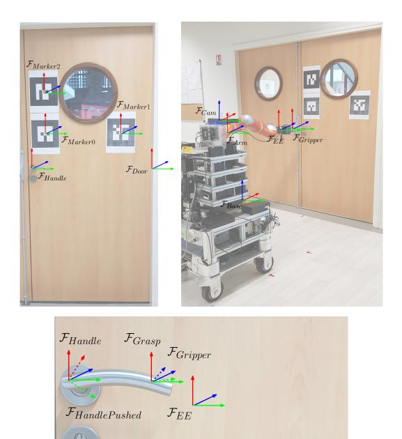
Figure D.1: Illustration of the different frames for the localization process.
