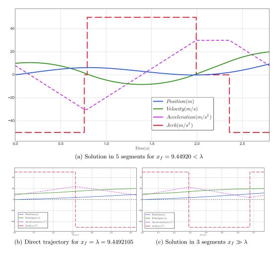
Figure 2.9: Major effects of discontinuities on the time representation of the optimal trajectory and its derivative.
