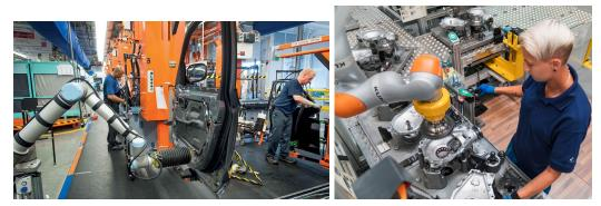
(a) A universal cobot used in car assembly production (b) LBR iiwa of KUKA cooperating with line. BMW employee in Dingolfing's factory.
