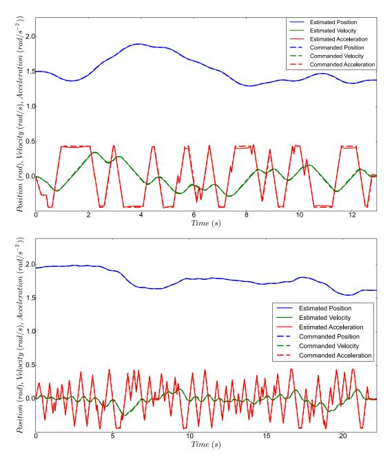
Figure 3.20: Evolution of angular trajectories during some visual servoing experiments. As the trajectory planner runs at 10Hz, trajectories are replanned multiple times while the robot is moving. Junction trajectories are used to smooth the trajectories switch.
