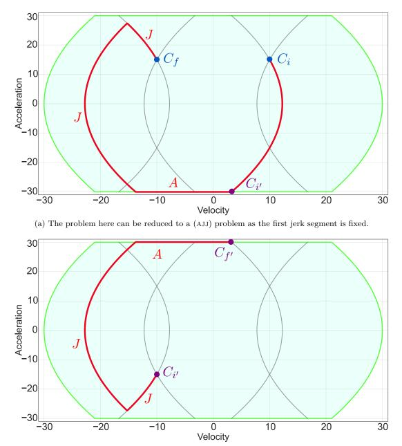
(b) The (AJJ) sequence presented in (a) can be transformed by symmetry according to the acceleration axis. The symmetric of  $C_{f'}$  becomes the  $C_{i'}$  of the (JJA) sequence, and the same can be applied to  $C_{i'}$  that becomes  $C_{f'}$  after transformation.
