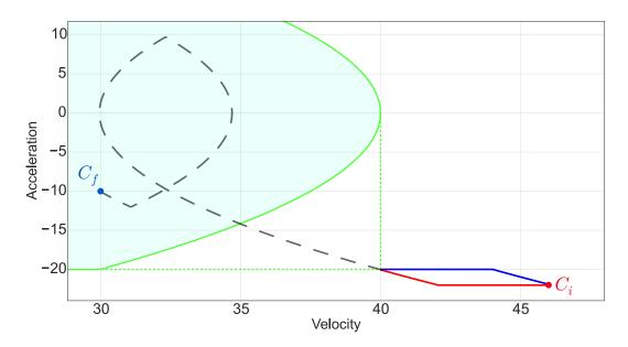
Figure 3.8: Our solution to reach  $\mathcal{D}$  here in red, and the one presented in [Kroger 2010, Zhao 2017] in blue (Sec. 3.2.5.1). We choose the following configuration:  $C_i = (0, -20, -22)$  and  $V_{max} = 40, A_{min} = -20$  so  $C_i$  belongs to A5.
