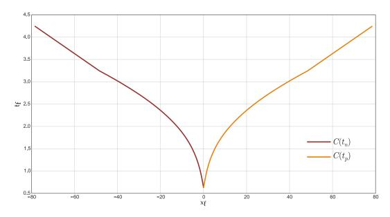
Figure 2.7: The optimal time solutions  $(t_f)$  versus the trajectory length  $(x_f)$ . A trajectory length of zero means the start and end positions are the same. For example, the trajectory with  $x_f = 0$  length is here associated to the direct trajectory of Fig. 2.4, and the null length is explained by the presence of symmetries.  $(J_{min}=-50, J_{max}=50, A_{min}=-30, A_{max}=30, V_{min}=-30, V_{max}=30, a_i=8, v_i=-5, a_f=8, v_f=5).$
