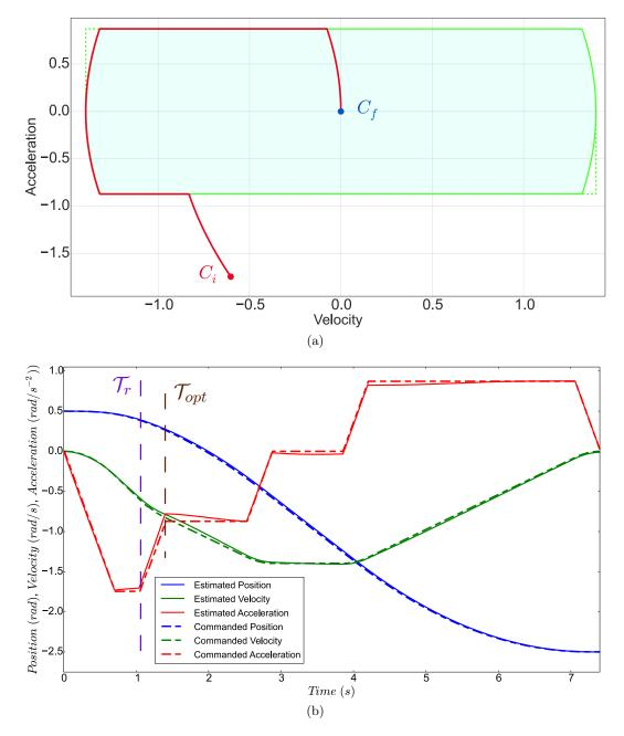
Figure 3.16: Acceleration bounds are decreased and the current configuration of the arm belongs to A2.  $T_r$  is made of a positive jerk segment reaching  $A_{min}$  at t = 0.7s.
