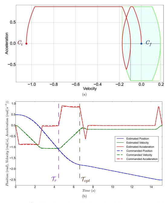
Figure 3.17: Speed bounds are drastically decreased, and the arm is in an invalid configuration belonging to A4. A new trajectory is computed to bring the system into  $\mathcal{D}$ .
