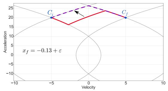
(b) Negative shortcut trajectory corresponding to the situation depicted by the brown circle on the time-optimal curve  $C_{opt}$  of Fig. 2.10. By increasing  $x_f$  we follow the lens shaped curve of  $C_{opt}$  until the direct trajectory depicted in purple here and by the purple circle in (a).
