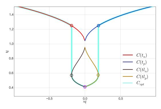
Figure 2.10: Shortcut trajectories introduce discontinuities in the time-optimal curve  $C_{opt}$ . The color circles are placed on the sides of the discontinuities that are depicted in the phase diagram in Fig. 2.11, 2.12.  $(J_{min}=-40, J_{max}=40, A_{min}=-30, A_{max}=30, V_{min}=-30, V_{max}=30, a_i=20, v_i=-4.99, a_f=20, v_f=4.99).$
