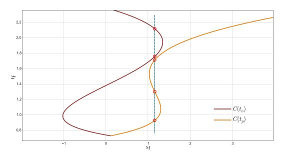
Figure 2.13: Curve exhibiting up to 5 solutions when initial and final velocities are shifted.  $(J_{min}=-40, J_{max}=50, A_{min}=-55, A_{max}=50, V_{min}=-40, V_{max}=70, a_i=-39.0, v_i=17.205, a_f=-39.0, v_f=-17.105).$
