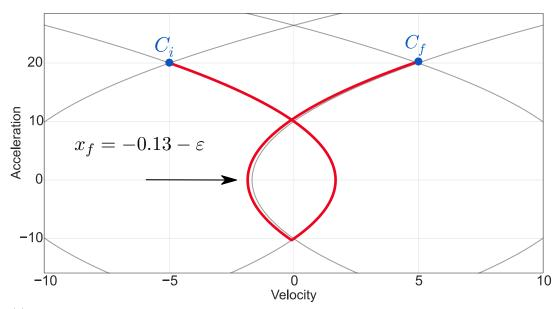
(a) Negative loop trajectory corresponding to the situation depicted by the red circle on the timeoptimal curve  $C_{opt}$  of Fig.2.10. If  $x_f$  is increased, the shape of the time-optimal trajectory change drastically (see (b)) as there is a discontinuity on  $C_{opt}$ .
