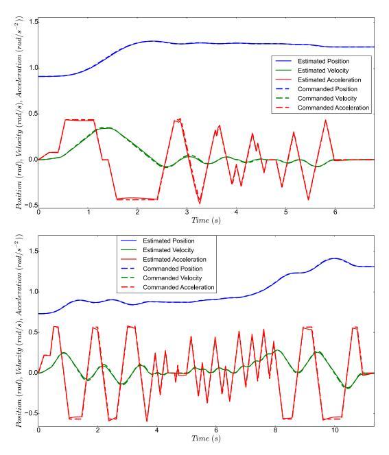
Figure 3.21: Evolution of angular trajectories during some visual servoing experiments. As the trajectory planner runs at 10Hz, trajectories are replanned multiple times while the robot is moving. Junction trajectories are used to smooth the trajectories switch.
