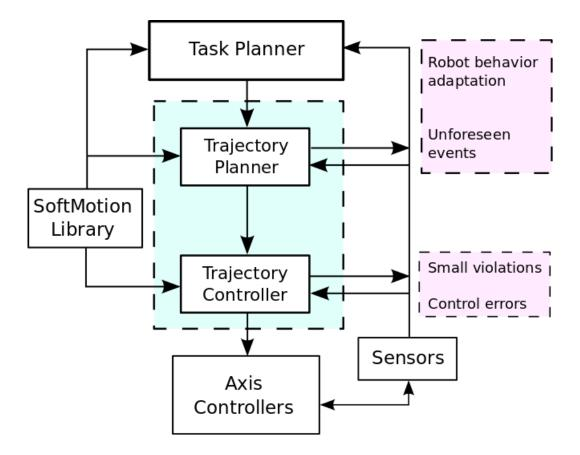
Figure 3.1: An architecture for Reactive Trajectory Control.
