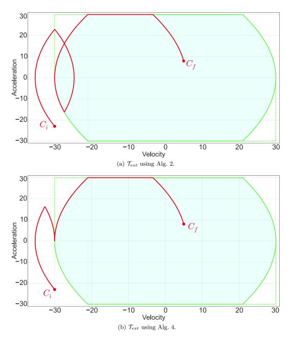
Figure 3.6: Configuration used :  $(J_{min}=-50, J_{max}=50, A_{min}=-30, A_{max}=30, V_{min}=-30, V_{max}=30, a_i=-23, v_i=-30, a_f=8, v_f=5, x_f=-400).$
