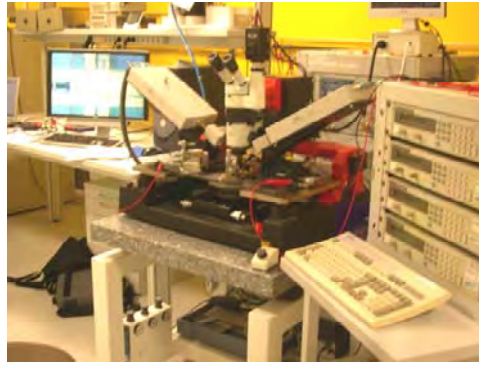
Figure 7. The experimental setup used for TBPF characterization
