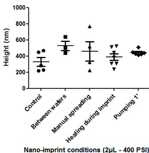
Figure 3.17.: Polyacrylamide thickness measurements by profilometry, depending on the nano-imprint conditions with NANONEX machine, corresponding to the deposition of a  $2\mu\text{L}$  solution volume. For the statistics corresponding to each dataset, see Table 3.2.
