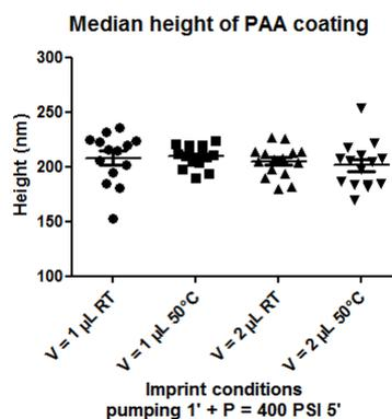
Figure 3.18.: Polyacrylamide thickness measurements by profilometry, depending on the thermal nano-imprint conditions with NANONEX machine, and the deposition of a decreasing solution volume. For the statistics corresponding to each dataset, see Table 3.3.
