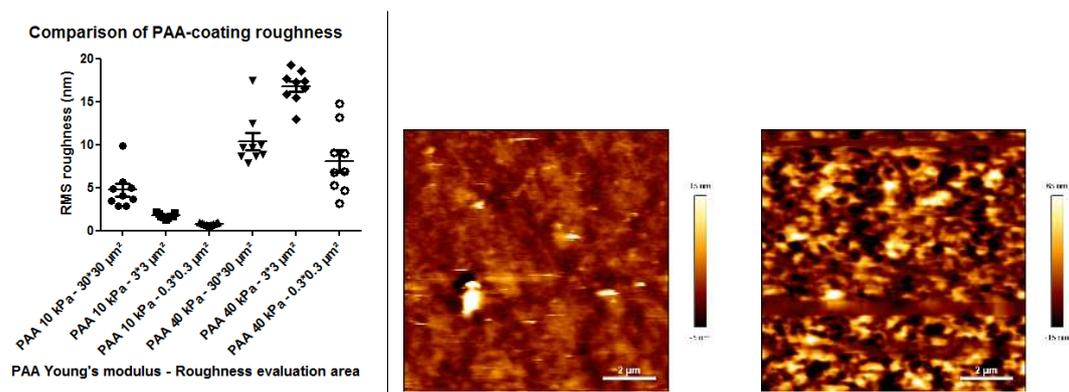
Figure 3.13.: Comparison of two polyacrylamide coating roughness with AFM (left), and the corresponding acquisitions for  $10*10 \mu\text{m}^2$  areas for Young's modulus value of 10 kPa (center) and 40 kPa (right). For the statistics corresponding to each dataset, see Table 3.1.
