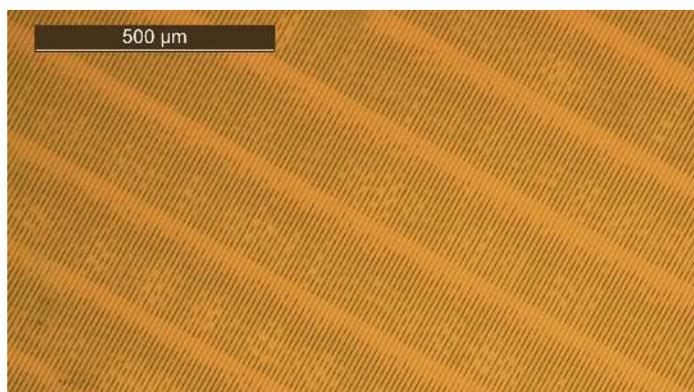
Figure 3.40.: Optical microscope observation of the center of the coverslip, 10x magnification. The sample was exposed with a dose of  $100 \text{ mJ}\cdot\text{cm}^{-2}$  in hard contact, and developed for 60 seconds in CD MF-26. Resist motifs discontinuities appeared periodically distributed.
