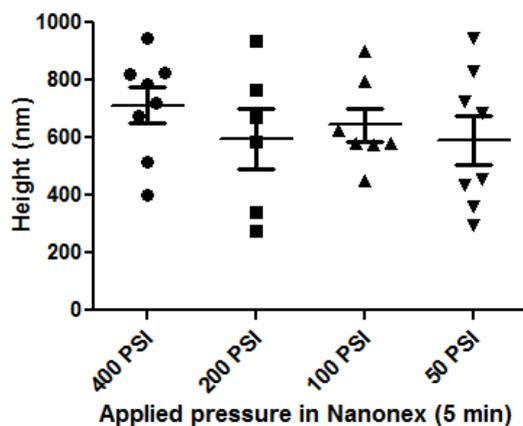
Figure 3.16.: Polyacrylamide thickness measurements by profilometry, depending on the applied pressure with NANONEX machine, corresponding to the deposition of a  $2\mu\text{L}$  solution volume.
