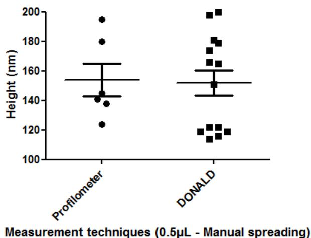
Figure 3.15.: Polyacrylamide thickness measurements performed by either profilometry or with DONALD setup, corresponding to the deposition of a 0.5  $\mu\text{L}$  solution volume.
