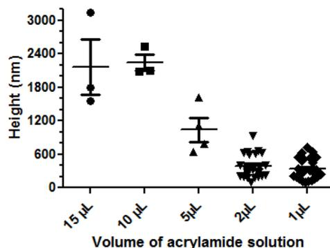
Figure 3.14.: Polyacrylamide thickness measurements by profilometry, corresponding to the deposition of a decreasing solution volume.
