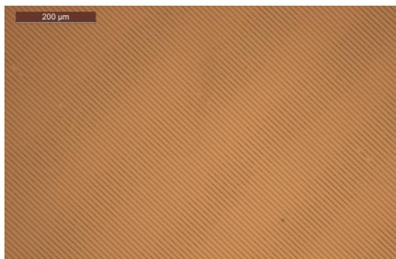
Figure 3.39.: Optical microscope observation of the center of the coverslip, 10x magnification. The sample was exposed with a dose of  $100 \text{ mJ}\cdot\text{cm}^{-2}$  and developed for 60 seconds in CD MF-26. Resist motifs appeared well-defined and continuous.
