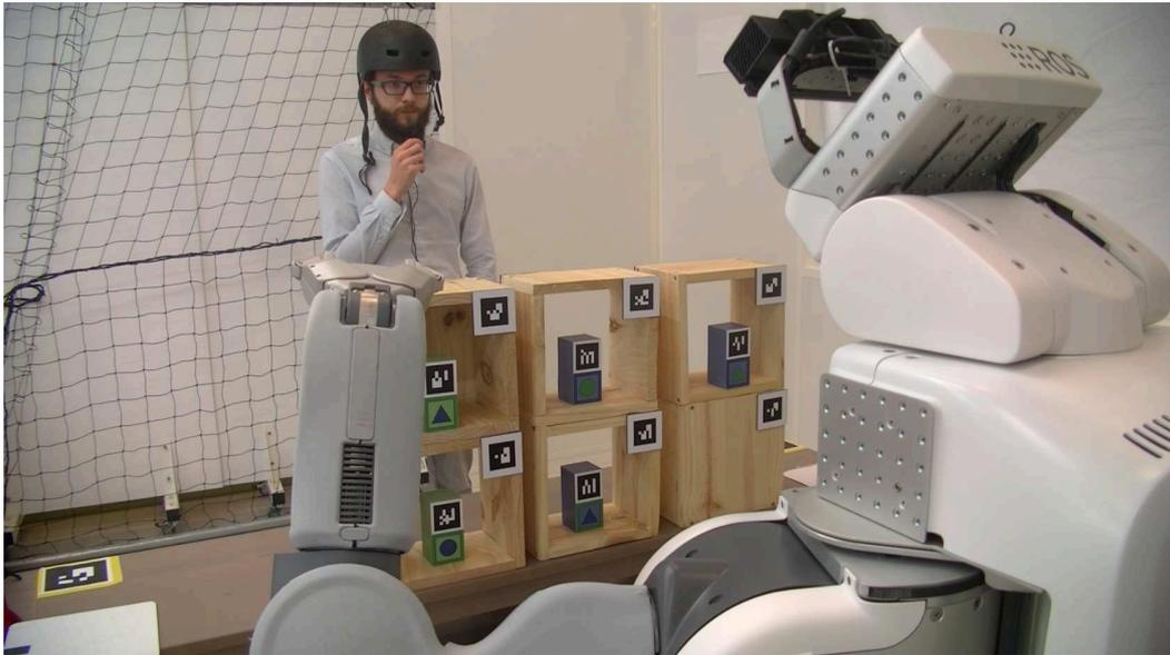
Figure 9.7: Initial configuration for both case studies. The top-right block is not visible, and thus unknown, by the human partner. The robot can not know if there is a block in the bottom-left compartment. All other blocks are known by both the robot and the human.
