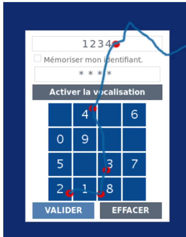
Figure 5.10: Retrieving the credentials by combining mouse movements and malicious screenshot
